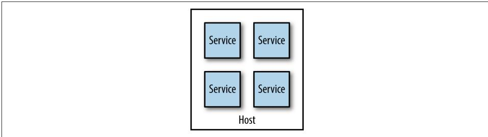
Figure 6-6. Multiple microservices per host
