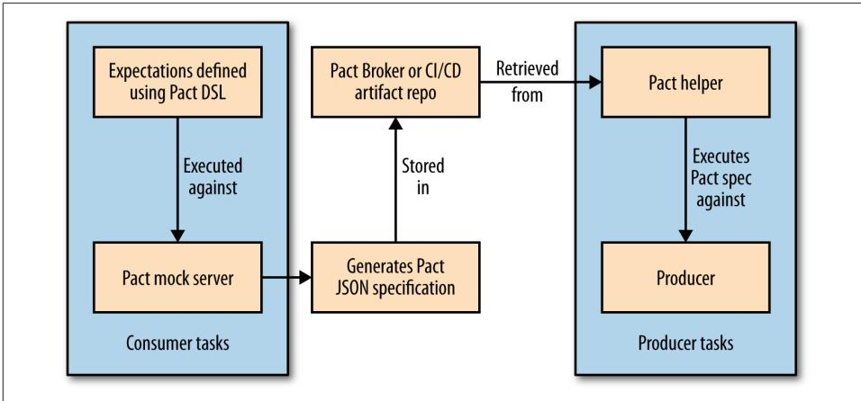
Figure 7-11. An overview of how Pact does consumer-driven testing
