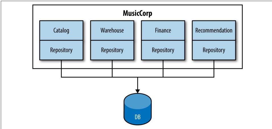
Figure 5-1. Splitting out our repository layers
