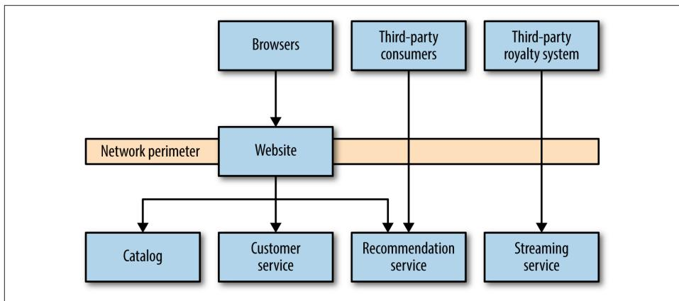
*Figure 9-4. A subset of MusicCorp's unfortunately insecure architecture*
