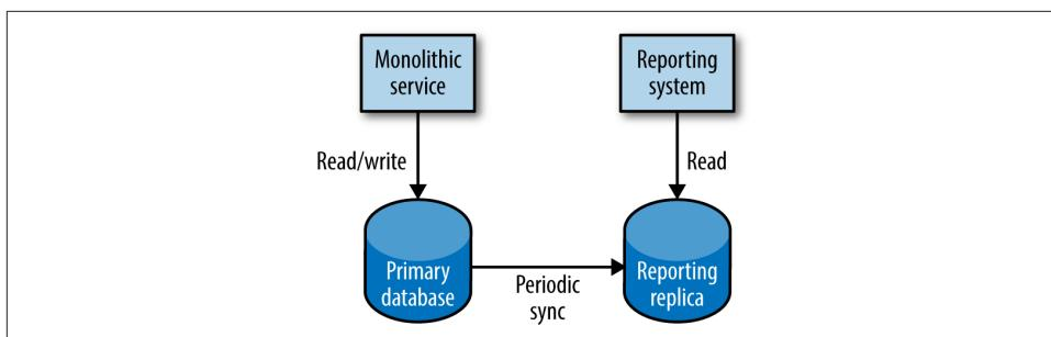
*Figure 5-12. Standard read replication*
