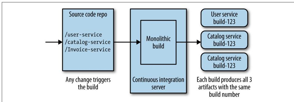
Figure 6-1. Using a single source code repository and CI build for all microservices
