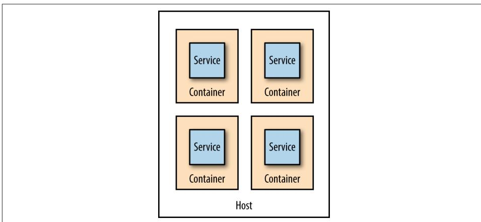
*Figure 6-10. Running services in separate containers*
