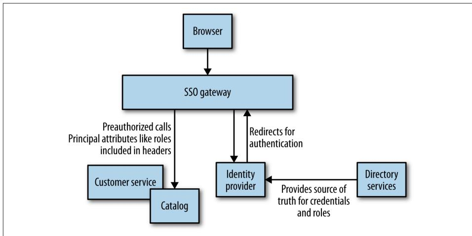
Figure 9-1. Using a gateway to handle SSO
