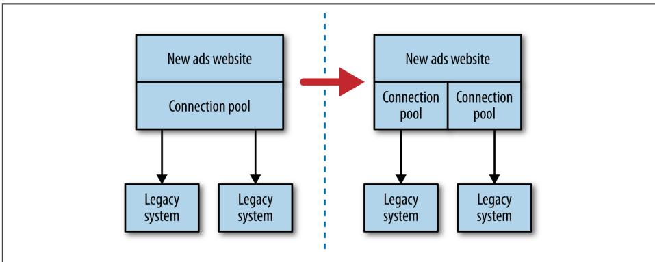
Figure 11-3. Using a connection pool per downstream service to provide bulkheads
