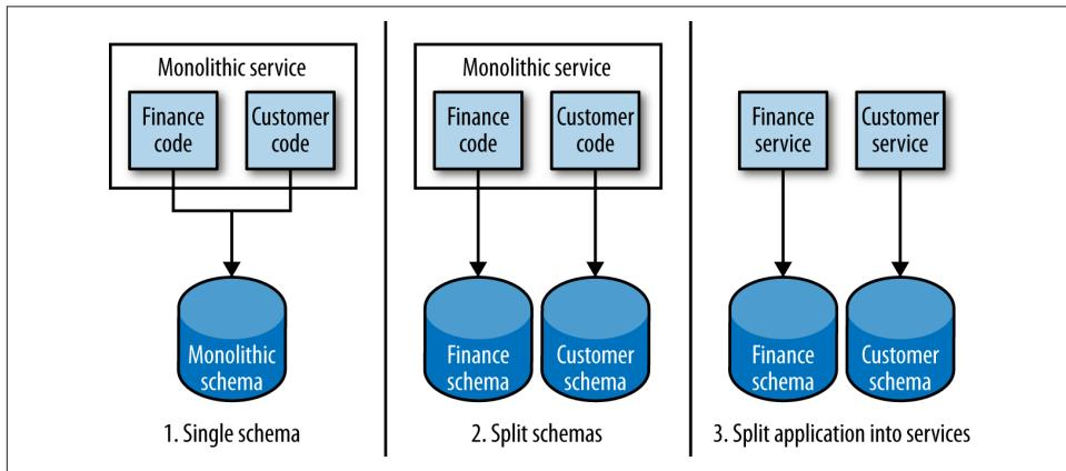
Figure 5-9. Staging a service separation
