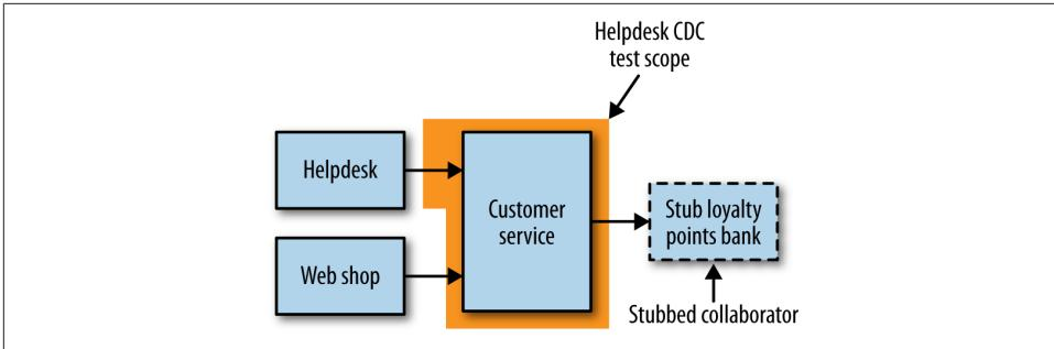
Figure 7-9. Consumer-driven testing in the context of our customer service example
