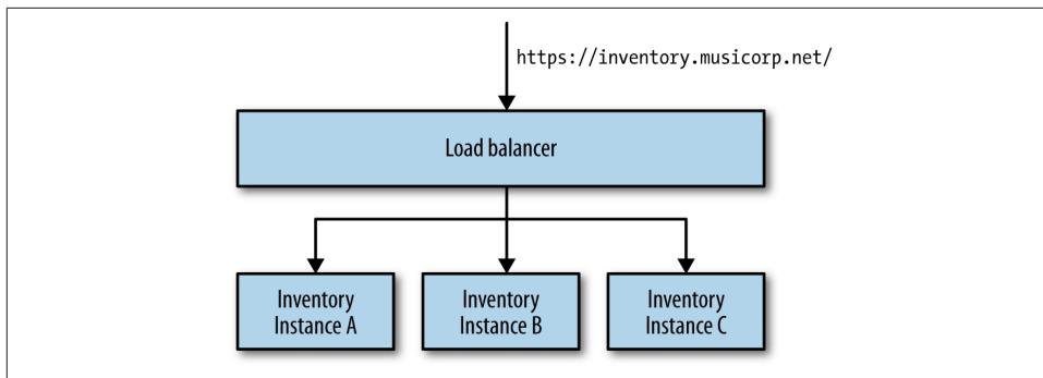
*Figure 11-9. Using DNS to resolve to a load balancer to avoid stale DNS entries*
