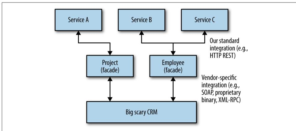
Figure 4-12. Using façade services to mask the underlying CRM
