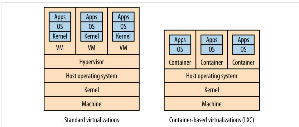
Figure 6-9. A comparison of standard Type 2 virtualization, and lightweight containers
