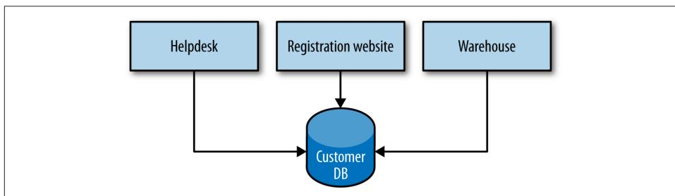
Figure 4-1. Using DB integration to access and change customer information
