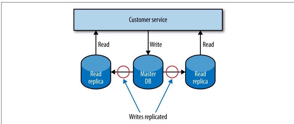
Figure 11-6. Using read replicas to scale reads
