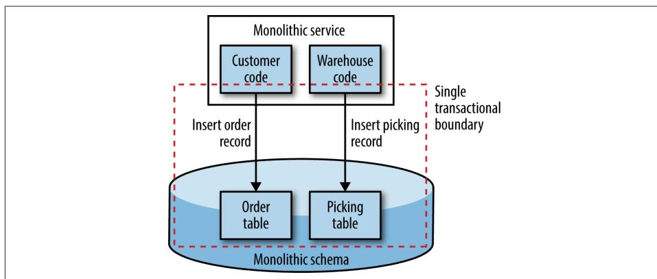
*Figure 5-10. Updating two tables in a single transaction*
