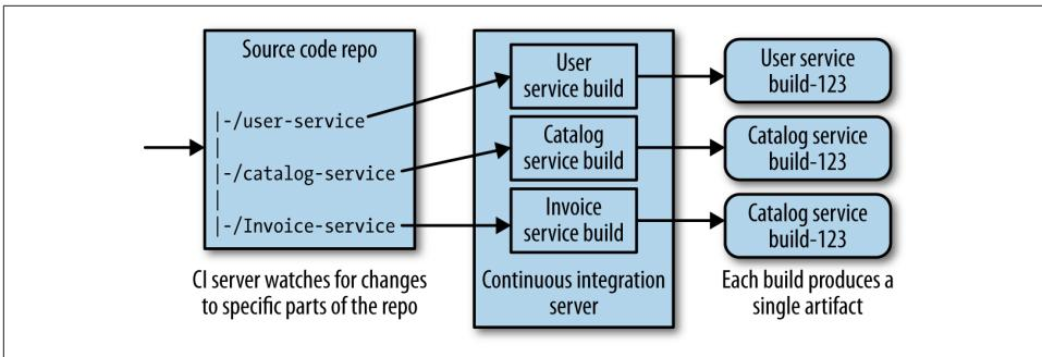
Figure 6-2. A single source repo with subdirectories mapped to independent builds
