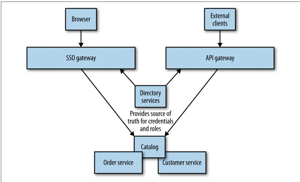
Figure 9-2. Using directory services to synchronize principal information between an SSO and an API gateway
