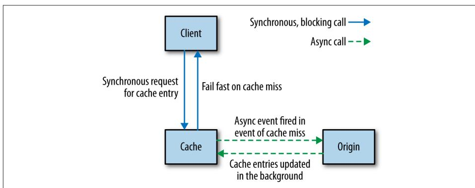
*Figure 11-7. Hiding the origin from the client and populating the cache asynchronously*
