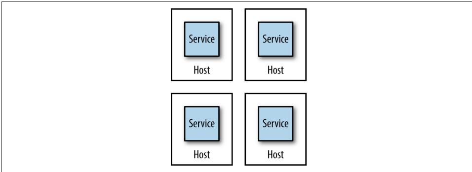
Figure 6-8. A single microservice per host
