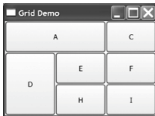
Figure 1-12. A sample Grid panel in action
