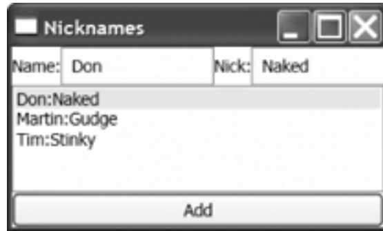
Figure 1-16. How a ListBox shows objects of a custom type with a data template
